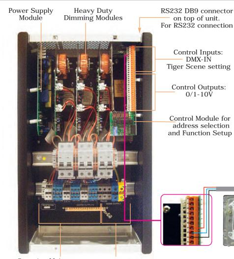
Outgoing Mains Circuit Connections Single or Three Phase Mains Input
