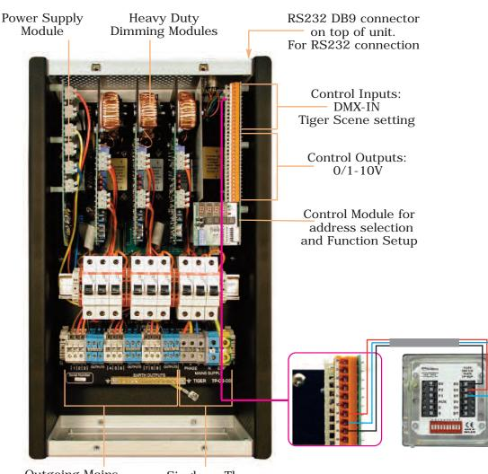
Outgoing Mains Circuit Connections Single or Three Phase Mains Input
