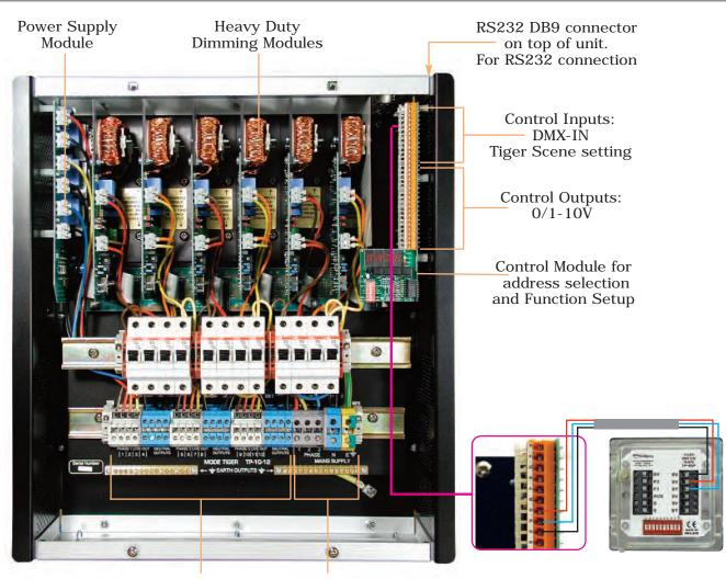
Outgoing Mains Circuit Connections Single or Three Phase Mains Input
