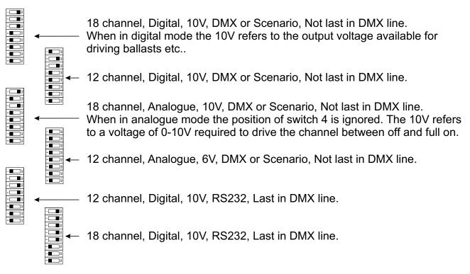
Maximum number of channels for DMX operation is 512. Maximum number of channels for Scenario operation is 99. In the event of a DMX or Scenario error the last level received will be maintained.
