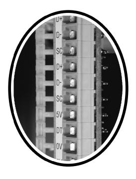
Lever operated screwless terminals as follows:-
