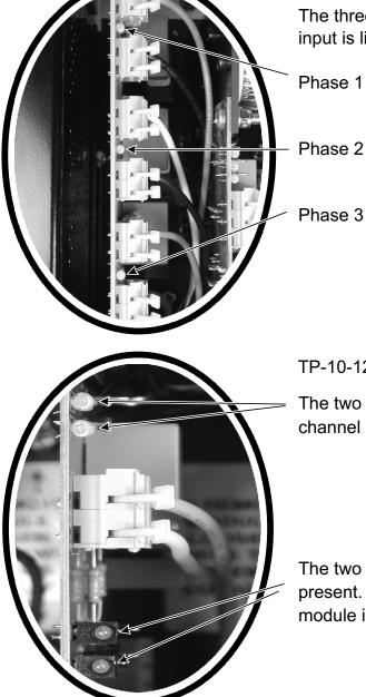
The three neons shown indicate when the phase input is live.
