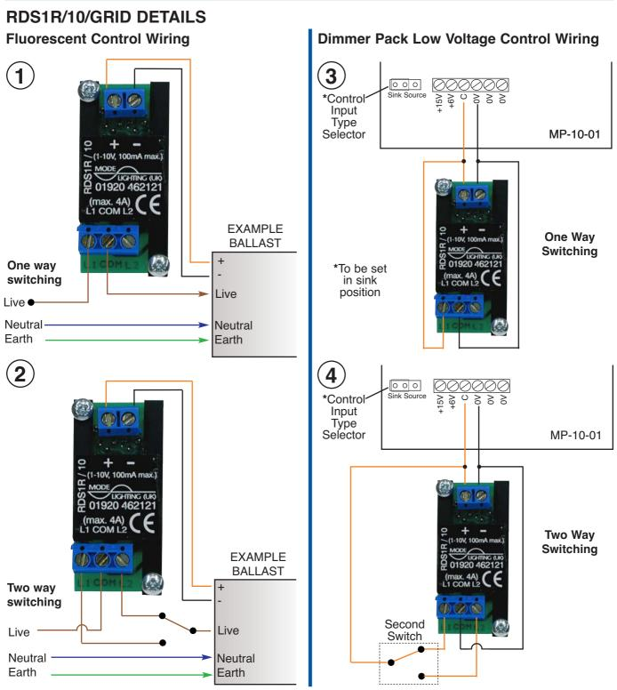
The 15K resistor supplied with the RDS1R/10/GRID is only required when controlling Mode dimmable power units MP-10-04 and MP-06-08. Please contact the Mode Lighting technical department for details.
