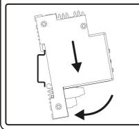
Modules must be installed within a suitable surface mount enclosure with integral DIN rail. Installation must be carried out by a qualified electrician in accordance with National Wiring Regulations and other applicable regulations. Compliance to EC EMC and Low Voltage Directives may be invalidated if not used or installed according to the published specification.
