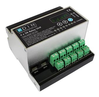
The Relay Contact Module is an ultra-compact DIN rail mounted unit with connections for four relay outputs and an M-BUS network. Each feed-through relay can switch 5 A with a maximum module load of 20 A.
